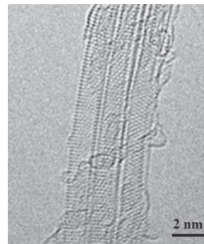
Figure 1. SWCNT image with high-resolution transmission electron microscopy (HR-TEM).
